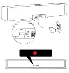
Step 3: Powering on the soundbar and enter into Bluetooth mode (Led indicator lights on blue)
